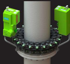
The conventional (hexagonal) nut remains on the bolt. Bolt strained torque-free with Bolt-Tensioner. Nut is turned by manually.
